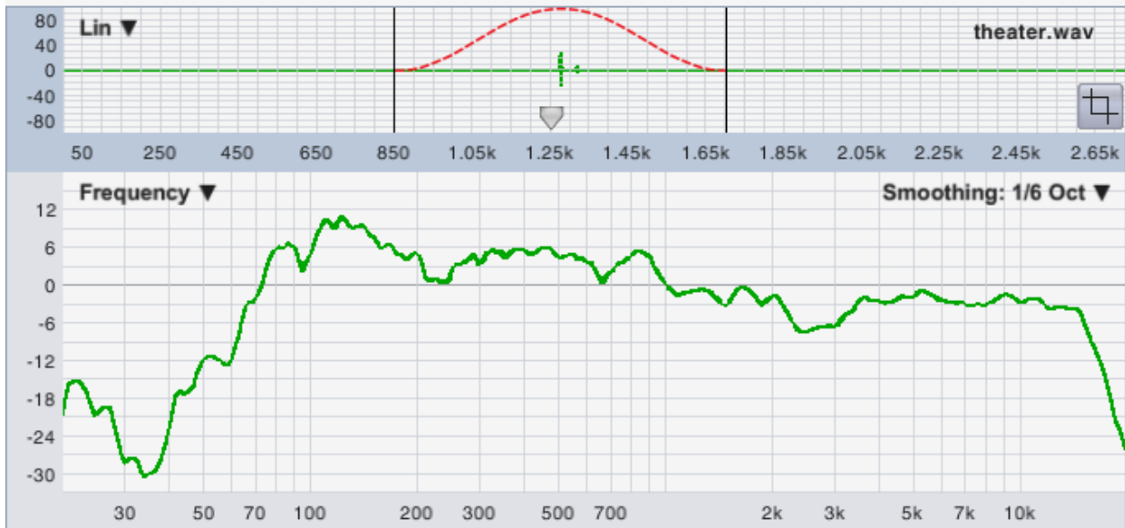
Figure 12: Moving the time 0 point and selecting a time range for display. The time range selected in the navigation pane applies to the Frequency graph as well as time domain graphs (Lin, Log or ETC). Note that Smaart uses a tapered data window when transforming any subset of the full IR time range. We've drawn the outline of a Hann window in red on the navigation pane of the "result" portion of the illustration above to help visualize this.
